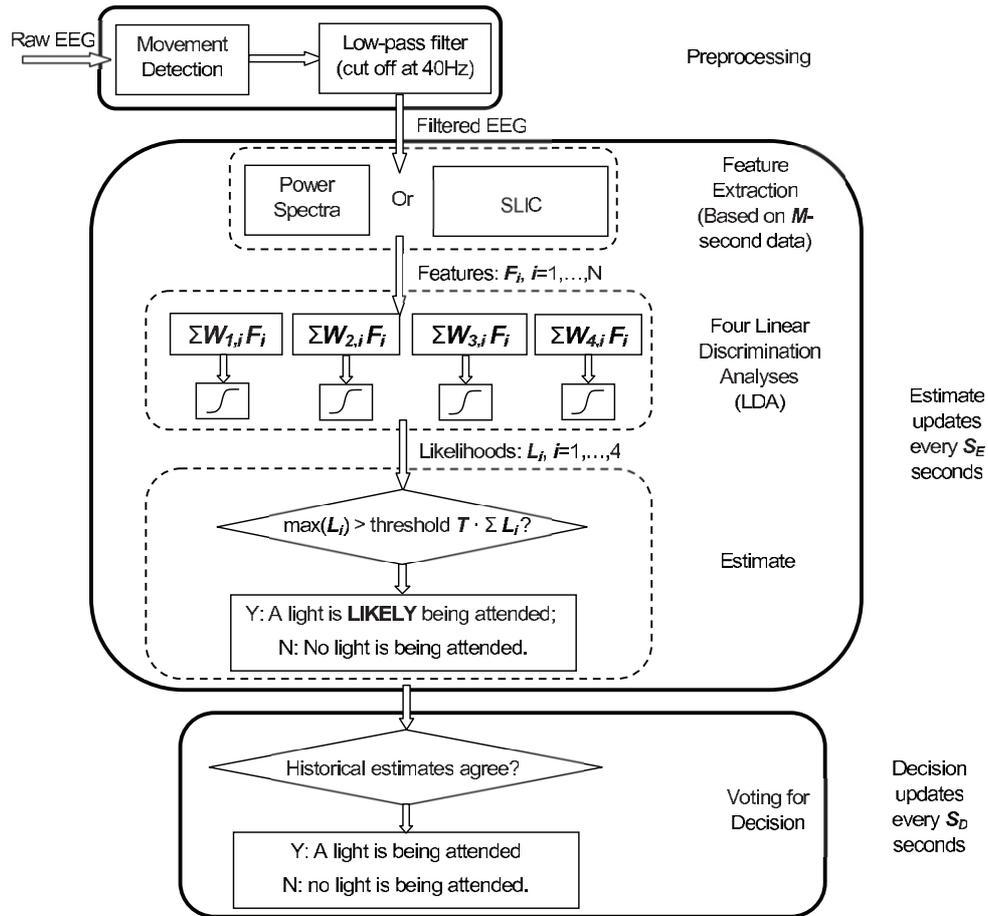
**Figure 3.** Flowchart of the data analysis process. It consists of preprocessing, feature extraction, LDA, estimation and decision stages. More details are discussed in the text.
