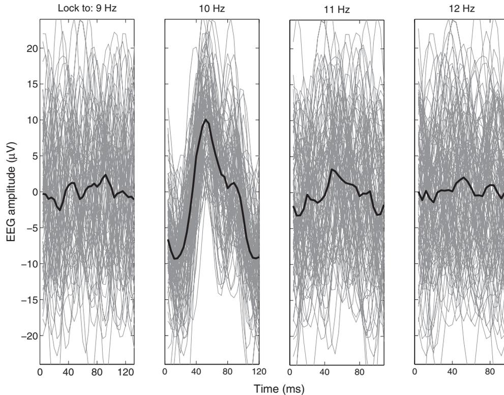
**Figure 2.** Example EEG traces (shown in gray curves) time-locked to the onsets of four different lights, flashing at 9, 10, 11 and 12 Hz, respectively. The EEG was recorded when the subject was attending to the 10 Hz light for 20 s. The black curves show the mean of the EEG traces.
